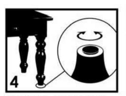
Some furniture come with optional height adjustment knobs underneath each leg. Turn this knob counterclockwise to raise the leg level or dockwise to lower the leg level.
