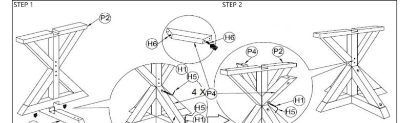
STEP 1A: Assemble Leg Section of Table
