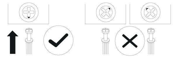
•Quickfit head should be in the centre of the cam lock wheen the two panels are joined.
