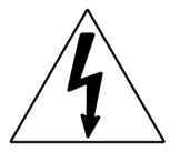
The lightning flash with arrowhead symbol, within an equilateral triangle, is intended to alert the user to the presence of uninsulated "dangerous voltage" within the product's enclosure that may be of sufficient magnitude to constitute a risk of fire or electric shock to persons
