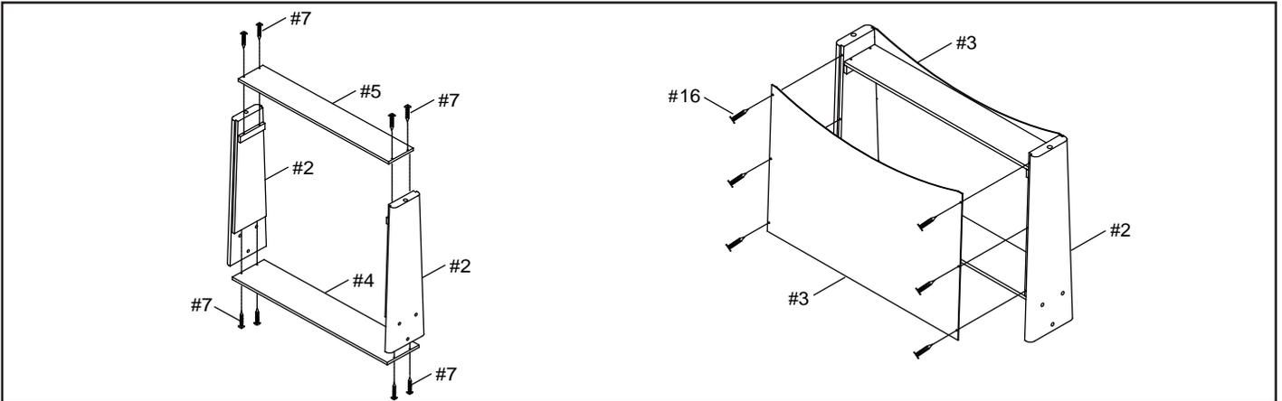
*Note: The Leg assembly may require two individuals, one to hold pieces, while the other inserts screws. TIP: If you hand insert all screws, on a single piece, into pre-drilled holes before tightening, it will help hold the pieces in alignment as you tighten the screws.*
