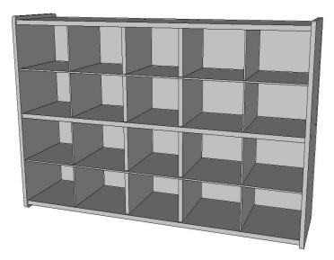
**Step 5:** Attach second **Side** piece using **(6)** supplied Hex screws and Allen wrench. Overhang on backs past Top, Bottom, and shelves will fit into deeper 3/8" back groove of second Side piece.
