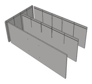
**Step 1:** Attach **Top, Bottom,** and **5/8**" **thick shelf** into a **Side** piece using **(6)** supplied **Hex screws** and **Allen wrench** provided. Back grooves in Top and Bottom, -cuts that go all the way through from short end to short end, align with 3/8" deep back groove in Side piece. Back grooves face inwards torwards middle of Side piece. Slots in 5/8" thick shelves also point torwards 3/8" deep back groove in Side piece.
