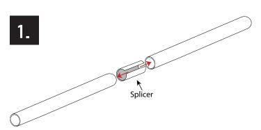
Use the splicer to join the two lengths of rail together. **NOTE:** For four foot kit, begin with step 2.
