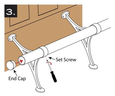
Secure the combination brackets in place with a set screw. Insert the end caps on each end of the rail. **NOTE:** Be sure to cover the seam of the joined rail with a combination bracket.
