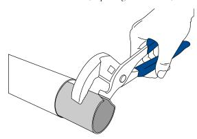
**TIP**: Use a wrench to crimp the splicer in order for it to fit inside the rail.
