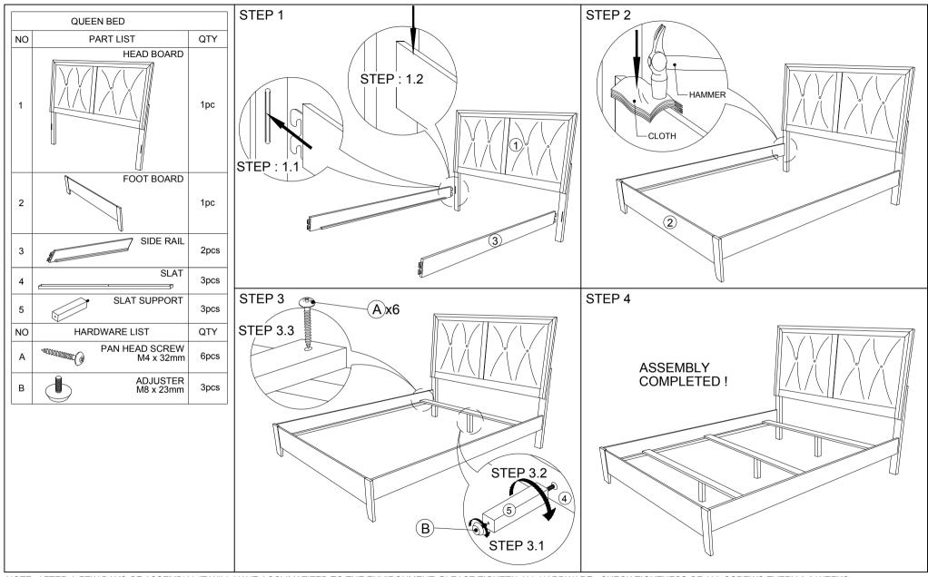
NOTE: AFTER A FEW DAYS OF ASSEMBLY, IT WILL HAVE ACCLIMATIZED TO THE ENVIRONMENT. PLEASE TIGHTEN ALL HARDWARE. CHECK TIGHTNESS OF ALL SCREWS EVERY 6-8 WEEKS.
