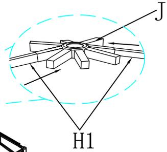
And assemble this part into the Top Connector J with the end of H1.
