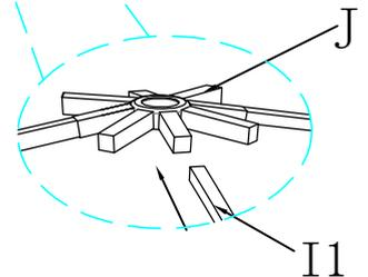
And assemble it to Beam D3 and the middle curtain bar E2 with the side of I2 by using screws BB
