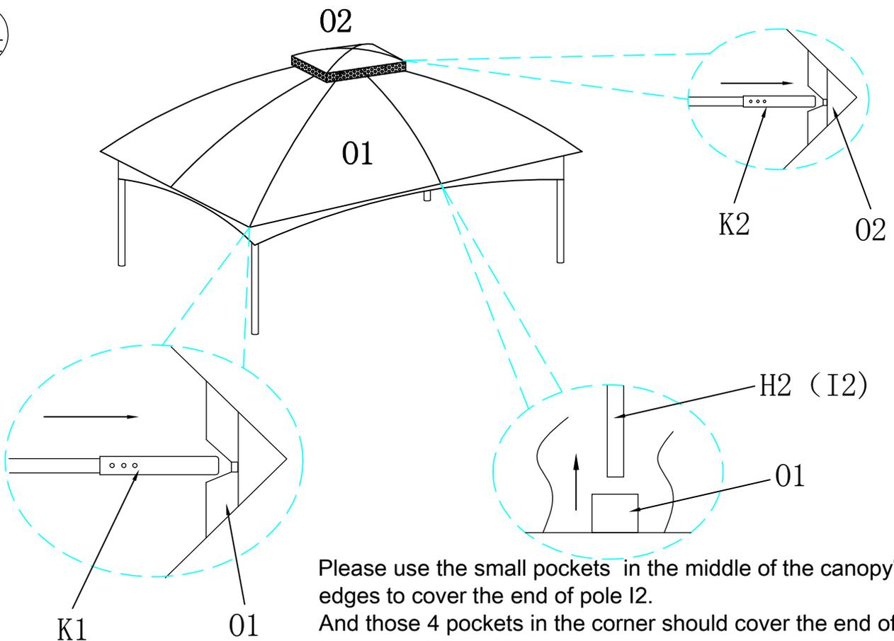
Please use the small pockets in the middle of the canopy's edges to cover the end of pole I2. And those 4 pockets in the corner should cover the end of 4 telescopic tubes K1.
