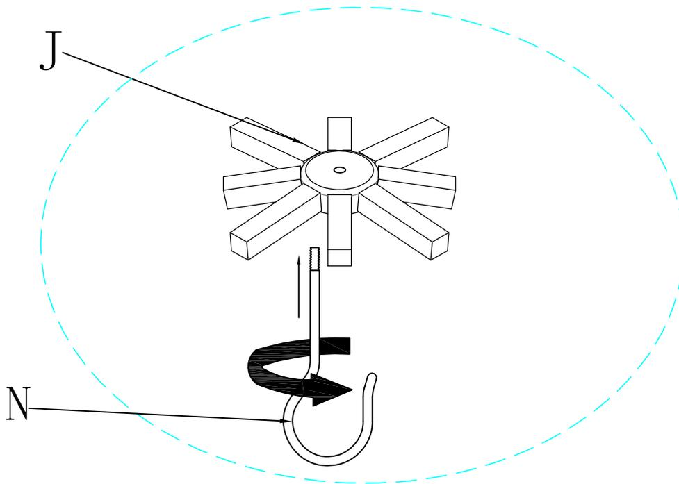
Connecting the Hook N to the Top Connector J.
