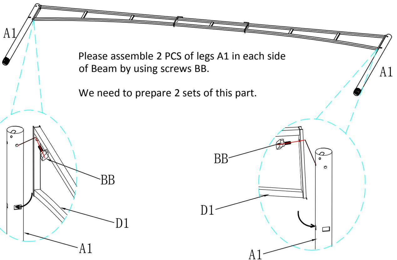
Please assemble 2 PCS of legs A1 in each side of Beam by using screws BB.
