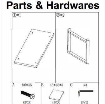
Step 1: Lay the Table Top(①) upside down onto a clean smooth surface such as carpet or cardboard. Align and fix two table legs (②) to the Table Top(①) with 8 pcs screw(A) by Allen Key(C).Do not fully tighten all bolts until all parts are in place.
