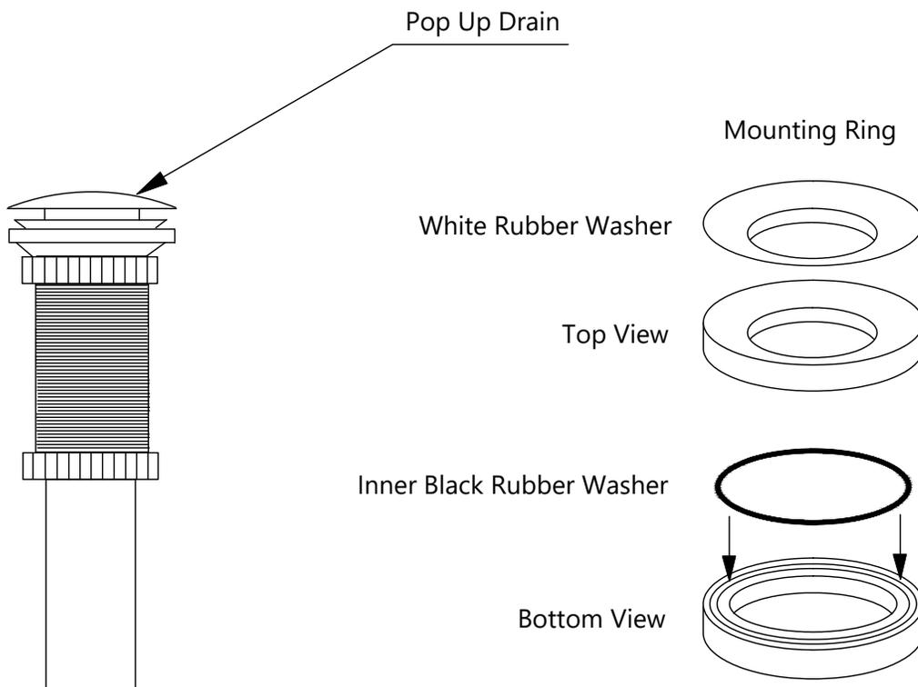
1. From above the countertop, insert the drain body into the 1 3/4" drain opening of your sink.
