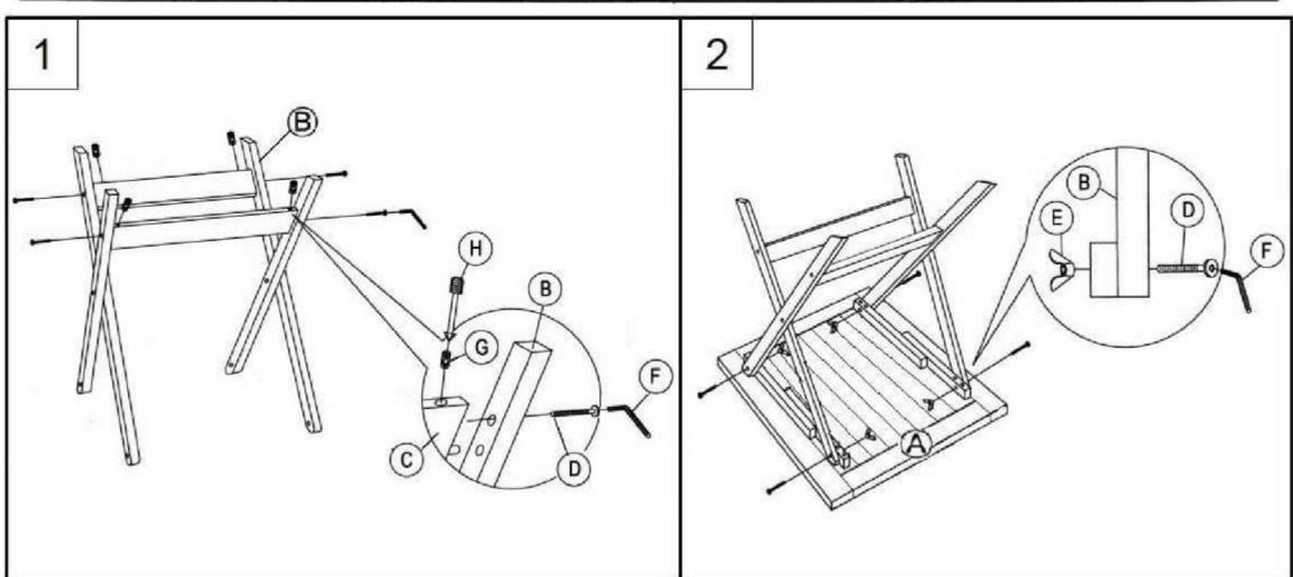
\* Do Not Tighten Any Bolt Until All Bolt Have Been Placed.
