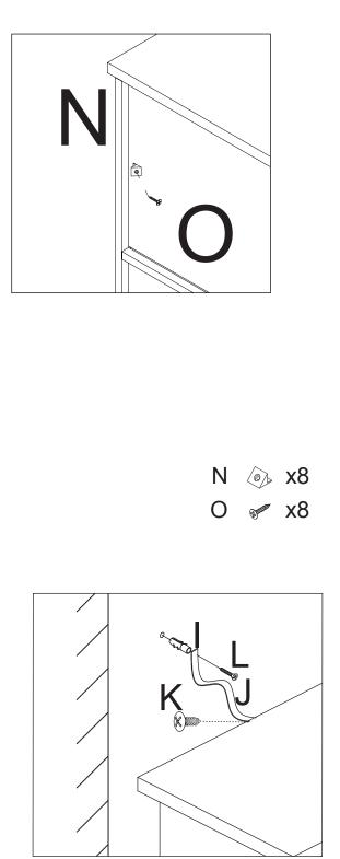
Drill hole on the wall with electrical drill, recommend size 5x40 mm Insert (I) into the wall with screw(L)
