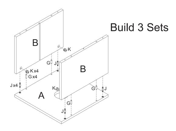
Insert the wooden dowels (G) and cam screws (J) into panel (A). Insert cam locks (K) into side panels (B). Attach side panels (B) to panel (A). Turn cam locks (K) clockwise to tighten.
