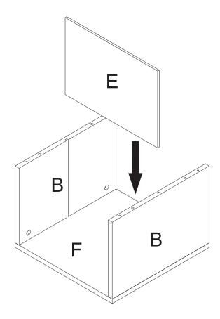
Slide the divider panel (E) into side panels (B).
