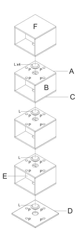
Insert connectors (L) into panels (A and D). Stack the cubes one by one.
