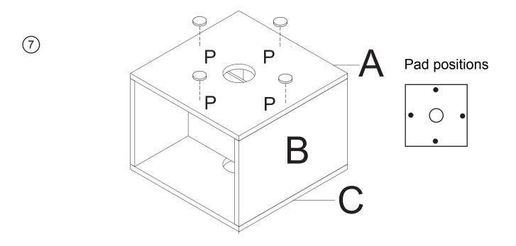
Remove the protective film from pads (P) and stick the pads onto panel (A), flat where shown.
