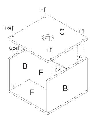
Insert the wooden dowels (G) into side panels (B). Attach the panel (C) to side panels (B) with screws (H).
