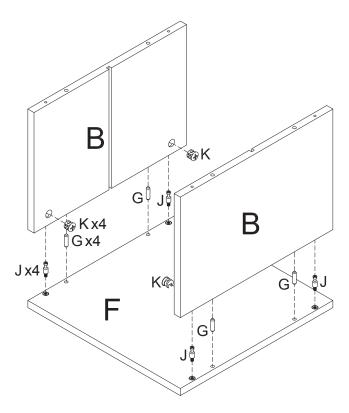
Insert wooden dowels (G) and fasten cam screws (J) into panel (F). Insert cam locks (K) into side panels (B). Attach side panels (B) to panel (F). Turn cam locks (K) clockwise to tighten.
