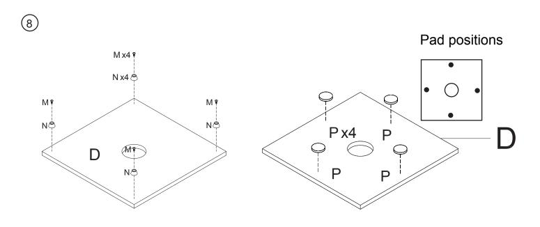
Attach the feet (N) to base (D) with screws (M). Then turn it over and stick the pads (P) onto panel (D), flat where shown.
