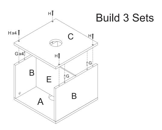
Insert the wooden dowels (G) into side panels (B). Attach the panel (C) to side panels (B) with screws (H).
