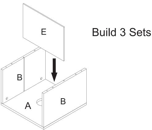
Slide the divider panel (E) into side panels (B).
