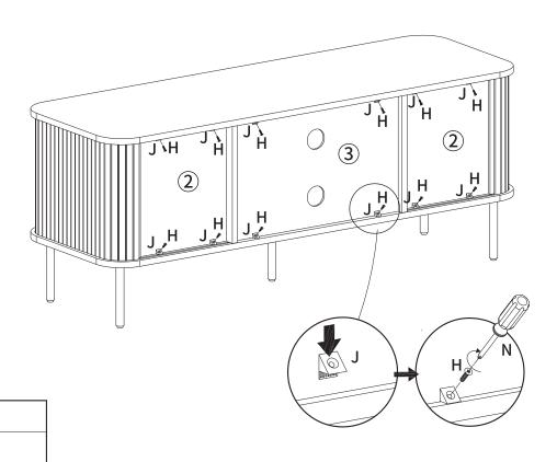
Insert (J) into the back of the cabinet, then twist Screw (H) to secure it.
