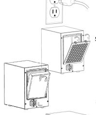
**Step 1:** Make sure the unit is unplugged before installing, removing any filters or maintaining the unit in any way, to prevent electric shock.
