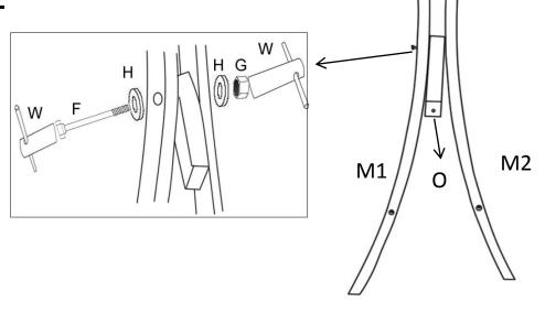
Attach Left Arch leg(M1), Arch stop(O), Right Arch leg(M2) together using Hardware(G,H,F) with Bucket Wrench(W).
