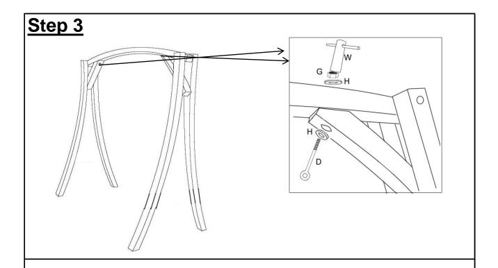
Attach the tail end of Arch stop (O) to the Arch connect(N) using Eye bolt(D) with hardware (H,G) and Bucket Wrench(W).
