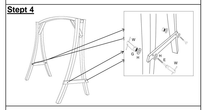
Attach Straight stop(P) to Arch leg(M1, M2) using hardware (G,H,E) with Bucket Wrench(W) .
