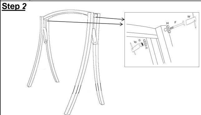
Attach Arch connect(N) between Arch leg(M1,M2),using hardware(H,F,G) with Bucket Wrench(W)
