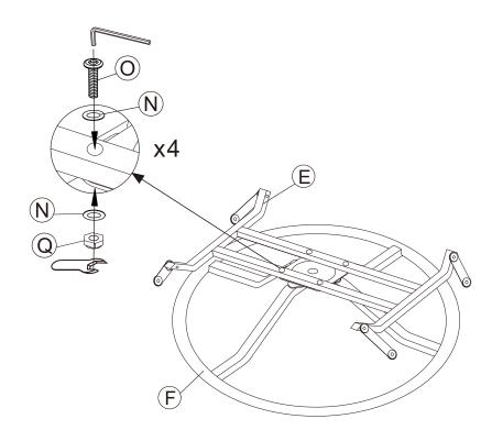
Place the turntable F flat on the ground, put the gasket N on the screw O, and assemble the support frame E and the turntable F according to the figure. Tighten the screw with the hex socket. (camber of support frame up)
