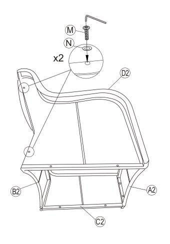
As shown in the figure, put a gasket N on the screw M and assemble it in the hole on the outside of the handrail (The handrails on both sides are assembled the same way.)
