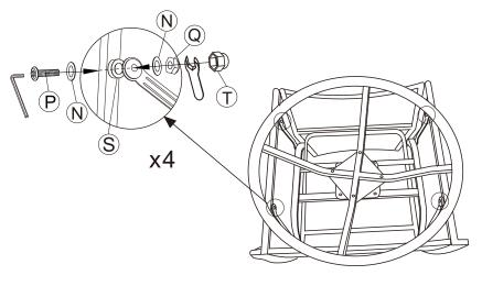
Place the bottom of the sofa assembled in step 4 upward on a clean plane, put gasket N over the screw P in the reserved hole at the bottom edge of the figure, assemble the four supporting feet of the metal support frame E, put on the plastic cushion S, gasket N, nut Q in order, and tighten the screw with the hex tool R and V. When assembled, the support frame is on the inside of the sofa.
