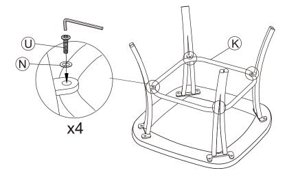
Place the gasket N over the screw U and fix the accessory K on the table foot H with the hex tool.
