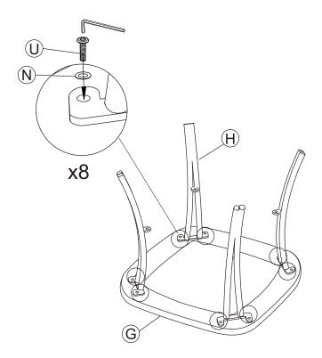
Place the table top G bottom up on a clean surface (the side with the assembly hole is the bottom) and align the hole of foot H with the assembly hole of the table top. Insert gasket N on screw U for assembly. Two screws per foot, a total of four feet.
