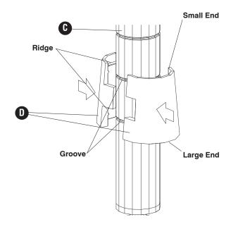
Connect the half-sleeves at the desired height for the lower shelf. Use lowest grooves for maximum capacity.
