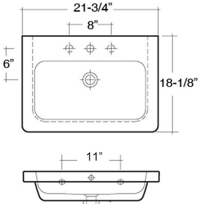
Dimensions of fixture are nominal and may vary within the range of tolerances established by ANSI Standard A112.19.2.2013. Dimensions and specifications subject to change without notice.
