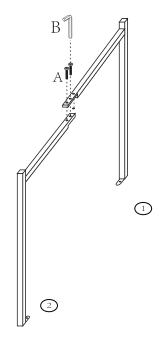
Join Half-Leg Sections (1 & 2) using Screw (A) as shown. (Note: for part (1) insert screws into first 2 holes closest to the horizontal end.)
