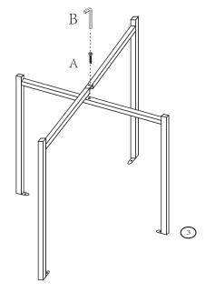
Place joined Leg Sections (1 & 2) from STEP 1 over Leg (3) as shown and align the screw holes. Next, use Allen Key (B) to drive Screw (A) to fasten the legs.
