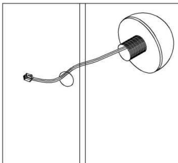
Make sure that you insert cables on bulb through prepared holes on board, suggest to insert once a time.
