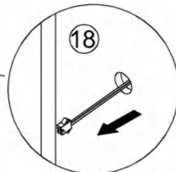
After passing the power cord of the bulb through the hole, stick the bulb onto the back panel
