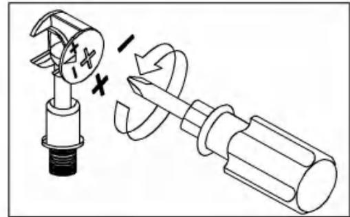
Disassemble along the direction of "-" sign
