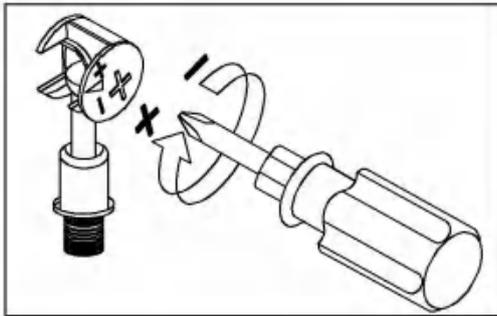
Use a screwdriver to lock in the direction of the "+" sign
