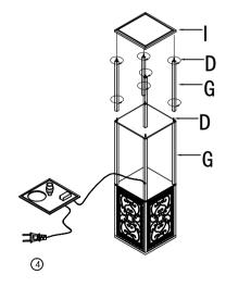
4. Screw and tighten long Pole(G) and Board (I) by screw(D)
