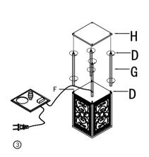
3. Screw and tighten long pole(G) and Board(H) by Screw(D)
