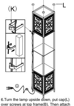
the clip(K) on the pole to secure the wire, your lamp is ready to use.
