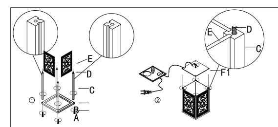
1. Carefully unpack all parts from the packaging and place them on a flat/smooth surface. Be sure to remove all the packaging materials from the lamp. Insert and tighten screw (A) into frame(B) and short pole(C). Then slide the shade(E) into short pole(C).
