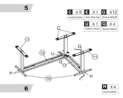
Note: Sync rods(12 and 13) and side brackets (10) installation direction
