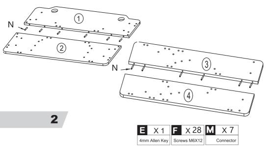
Note: The horizontal bar on the connector should be perpendicular to the seam of the table panel splice
