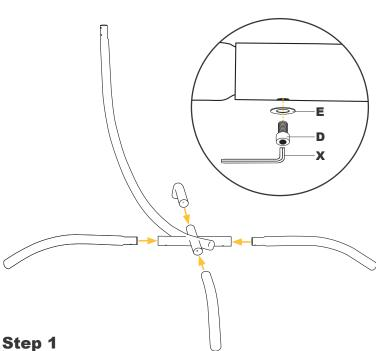
Slide Leg (C) into Bottom Pole (B). Align the holes on the underside of each piece. Hand-tighten Bolt (D) and Washer (E). Repeat until all legs are attached. Tighten all bolts using Hex Key (X).
