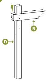
▶ Slide the Post Arm (B) down the Post (D) from the top as illustrated. Orient correctly to receive newspaper.
