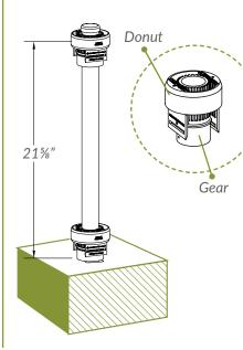
NOTE: Check that the pipe is level in both directions at about 6" intervals as you pound the pipe into the ground. Usually, after the pipe is about 18" into the ground, the trajectory of the pipe is established,
