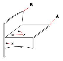
STEP 2 Connect the part from step 1 and right frame C with bolt N with allen key
