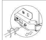
This is used to adjust the door panel in the left and right direction.
