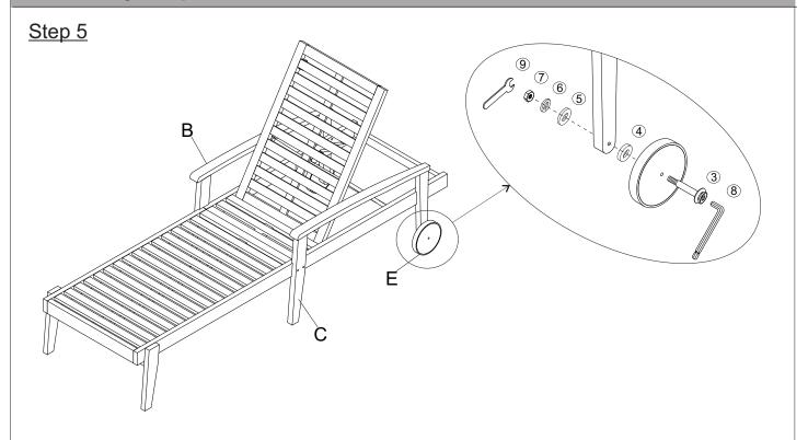
With the help of your adult partner, attach Wheels (E) to Right Leg Panel (C) using Wheel Bolt ( $\widehat{3}$ ), Washers ( $\widehat{4}$ ), Washers ( $\widehat{5}$ ), Spring Washers ( $\widehat{6}$ ) and Nuts ( $\widehat{7}$ ) with Allen Wrench ( $\widehat{8}$ ) and Wrench ( $\widehat{9}$ ) in the sequence as shown above. Repeat the same process with remaining Wheel (E) and the Left Leg Panel (B). **Do not fully tighten the Bolts**.
