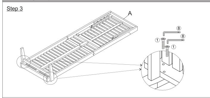
With the help of your adult partner, flip the assemble in step 2. Then attach Front Leg Panel (D) to Foldable Seat Panel (A) using Bolts (1) with Allen Wrench (8) as shown above. **Do not fully tighten the Bolts.**
