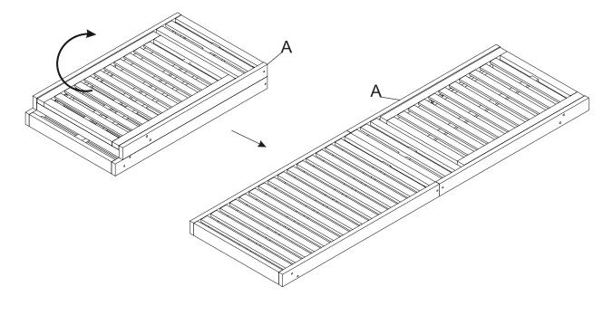
Unfold the Foldable Seat Panel(A) as indicated by the arrows.
