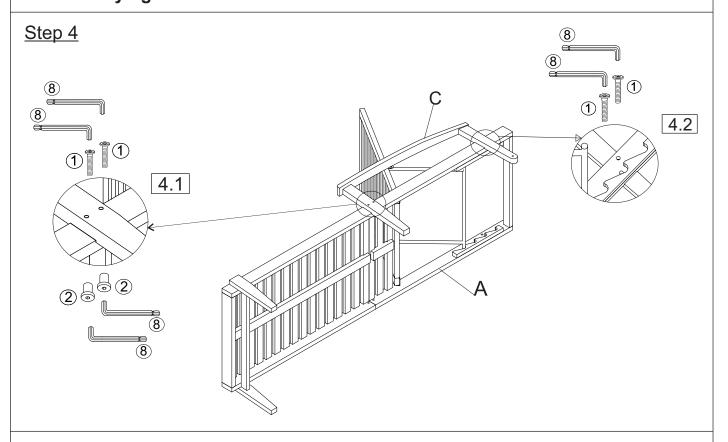
4.1) With the help of adult partner, attach the Left Leg Panel (C) to Foldable Seat Panel (A) using Bolts (1) and Sleeve Nuts (2) with Allen Wrench (8).
