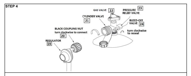
4. Turn the Cylinder Valve (21 ) on the tank in a clockwise direction to TURN OFF SUPPLY of the LP Gas supply .
