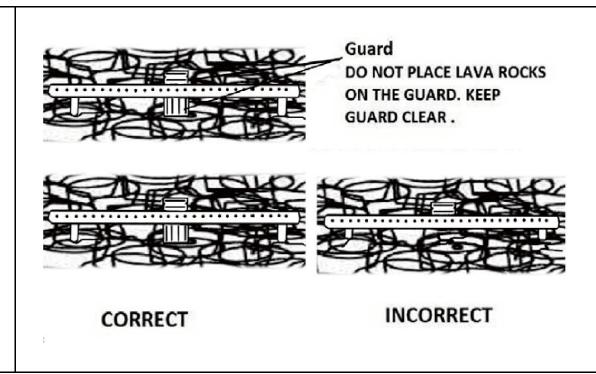
To ensure proper function, the Guard (01) on the Burner (08) should never have lava rocks (A) covered over it.
