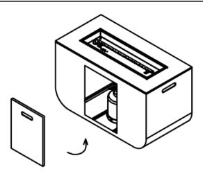
5. Replace and Close the Door (D) back to the Mainframe of the Fire Table / Column (C).
