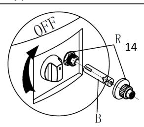
6. Remove the Electronic Ignitor Cap (14) on the electronic Ignitor (14) by unscrewing and slide the Battery (B) into the battery slot (14).
