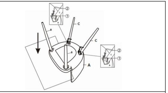
Attach Back Legs(C) to Chair Body(A) using Bolts(1) with Allen Key(2) as pictured above.
