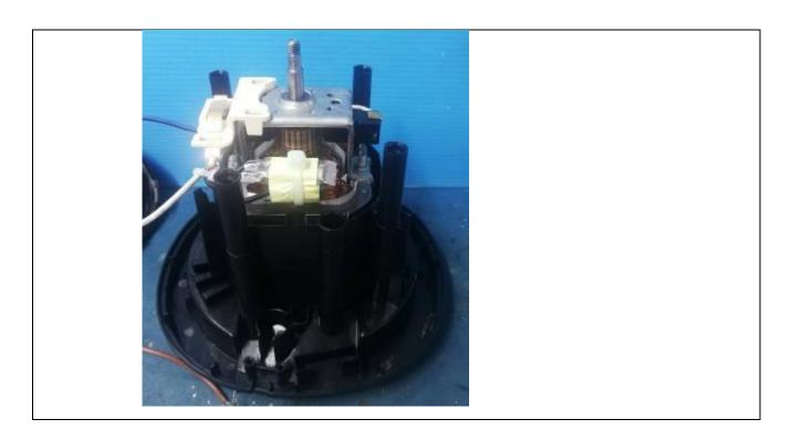
Details of: Motor KH76/20-Q with motor thermal protector
