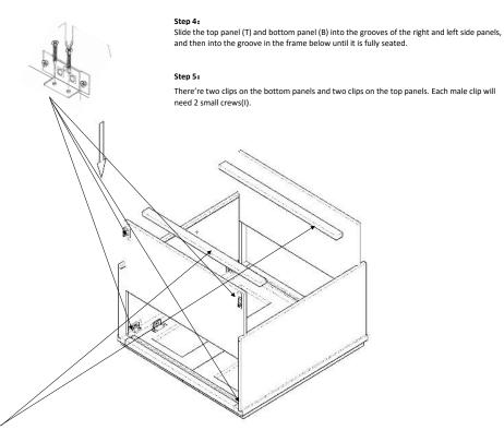
\*\* The two optional hanging bars are included, These are to be installed at the top & the biottom of the inside of the cabinet prior to mount to wall.
