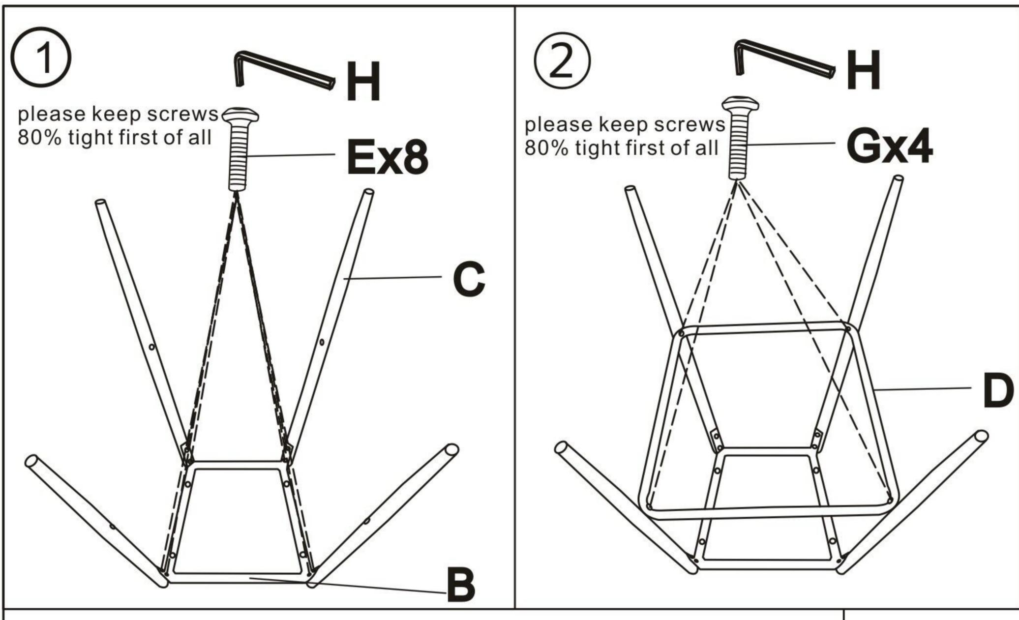
please put the legs into flat platform, then after adjustment, keep screws 100% tight finally.
