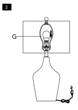
Step2 Insert the bulb( G) into the socket(C).
