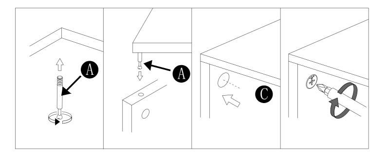
Read each step carefully before starting. It is very important that each step of instruction is performed in the correct order. If these steps are not followed in sequence, assembly difficulties will occur.
