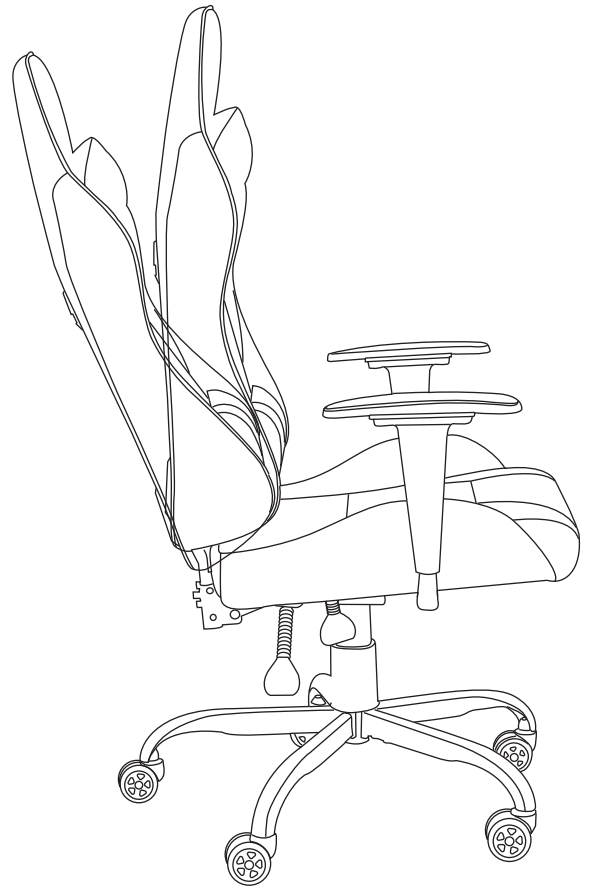
Counterclockwise rotation Rocking angle 10-30°
