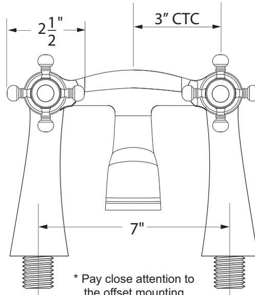
\* Pay close attention to the offset mounting legs. Although the faucet is a 6" spread, the mounting legs install into a 7" spread.
