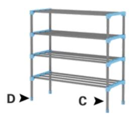
**Step 6**Install the top shelf stopper by using four C and two F.
