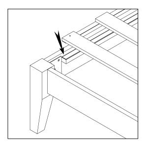
Velcro the ends of slat to the cleats of side rail
