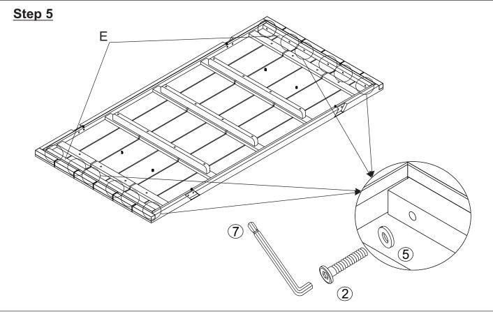
Attach the Second Support Bar (E) to the Side Table Top (A) and Middle Table Top (B) using Bolts (2) and Washers (5) with the Allen Wrench (7) as shown above. **Do not fully tighten the Bolts.**
