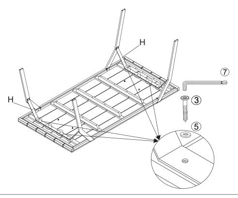
Secure the Connector Bar (H) to the Side Table Top (A) and Middle Table Top (B) using Screws (3) and Washers (5) with the Allen Wrench (7) as shown above. **Do not fully tighten the Screws**.
