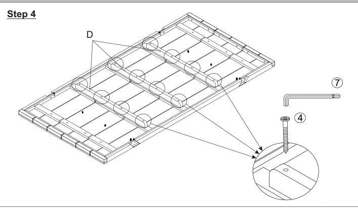
Attach the First Support Bar (D) to the Side Table Top (A) and Middle Table Top (B) using Screws (4) with the Allen Wrench (7) as shown above **Do not fully tighten the Screws**.
