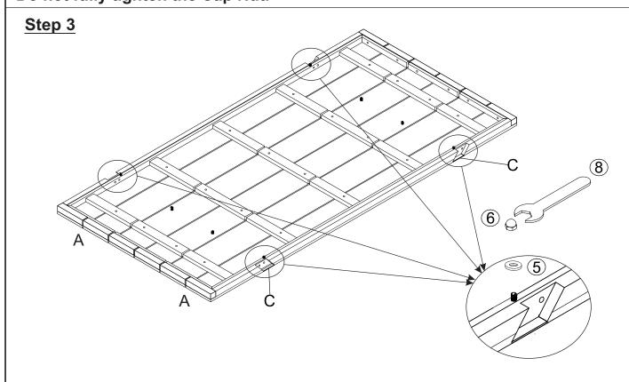
With the help of your adult partner, position the Side Table Top (A) to the Bar © using Cap Nuts (6) and Washers (5) with the Wrench (8) as shown above. **Do not fully tighten the Cap Nut.**
