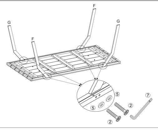
Attach the First Leg (F) and Second Leg (G) to the Side Table Top (A) (assembly from step 5) using Bolts (2) and Washers (5) with the Allen Wrench (7) as shown above. **Do not fully tighten the Bolts.**
