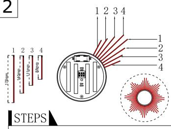
Rotate the aluminum tube clockwise and fix it on the lamp body as shown in the figure: 1,2,3,4-4,3,2,1 cycle sequence
