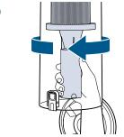
Twist cyclone left and pull down to remove from tank.
