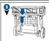
Check the air passageway on the bottom of your vacuum. Remove the bottom cover and the brush. Remove any debris.
