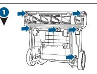
Unplug vacuum, turn over and unscrew six (6) Philips head screws to remove the bottom cover. Lift brush straight out.
