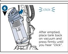
Clean cyclone with warm water and mild detergent. Let cyclone completely dry before replacing. To replace, fit into place and twist to the right.
