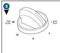
Turn the dial on the foot of the vacuum to the desired setting. If the dial is difficult to turn, tilt the vacuum back slightly to take the weight off the foot while turning.
