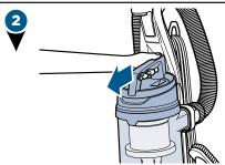
Press the tank release button and pull out to remove dirt tank.
