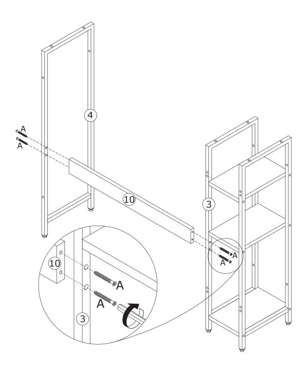
Fix part 3 and 4 to board 10 with screw(A) as shown.
