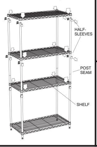
6 Set the unit into place and adjust the levelers at the bottoms of the posts until shelves are level in both directions.
