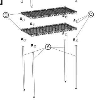
To build the four corner posts, screw the (A) Lower Posts (with levelers) onto the (B) Upper Posts (with plastic caps). Hand tighten.
