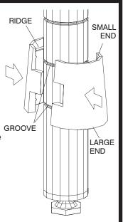
3 Stand a ① Shelf on end, and from the BOTTOM side of the shelf (the bottom side is recessed), slide the TOP end of a post through a corner hole until the half-sleeves are seated in the corner hole. Repeat with remaining posts.
