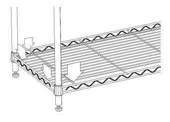
Snap half-sleeve sets onto all four posts at the desired height for the NEXT shelf. Lower this shelf into position and press until fully seated. Install the third and fourth shelves in the same manner, with both shelves mounted ABOVE the post seams.
