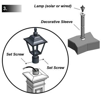
The decorative sleeve should sit flush on the ground leaving two inches of pipe exposed at the top. Connect the wiring and secure the lamp to the post. For solar lights simply secure the lamp to the post.
