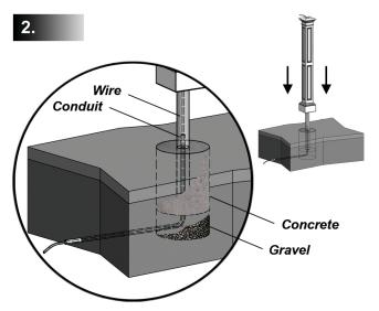
For hard-wired installations thread UF rated wire through the pipe and into the conduit. The conduit can be buried beside the post or directly in the center of the concrete footing leaving 6 inches exposed above ground. Outdoor wiring should be buried in conduit 18 to 24 inches below ground.
