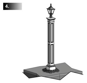
Remember to leave plenty of extra wire to reach the circuit-breaker panel inside the house. All outdoor wiring should be installed according to local electrical codes and inspected by a licensed electricians. To complete the installation you can back fill dirt around the base of the lamp post.
