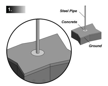
For solar lamp installations simply dig a hole approximately 15 inches deep and set the steel pipe in place leaving 74 inches above ground. Fill in the hole with concrete. For added stability dig a deeper hole and add 6 inches of gravel. This improves drainage and helps prevent heaving from frost.
