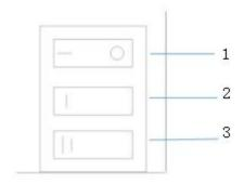
1. Flame switch - Switches flame effect and power on/off
