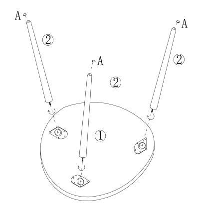
Assemble unit on carpet or other soft surface to avoid damage
