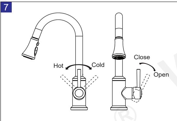
7 Lift the handle up, the cartridge will be activated allowing water to flow. The water flow will increase by continuing to rotate handle. By rotating the handle to the right, the water temperature will decrease to cold flow only. By rotating Handle to the left, the water temperature will increase to hot only.
