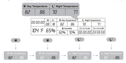
When the first value is less than the second value under the symbols " \* Day Temperature " and " \* Night Temperature ", it means heating mode.
