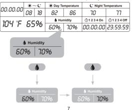
Continue to press " • ", the value in the humidity control setting area will stop flashing and the set value will take effect immediately.
